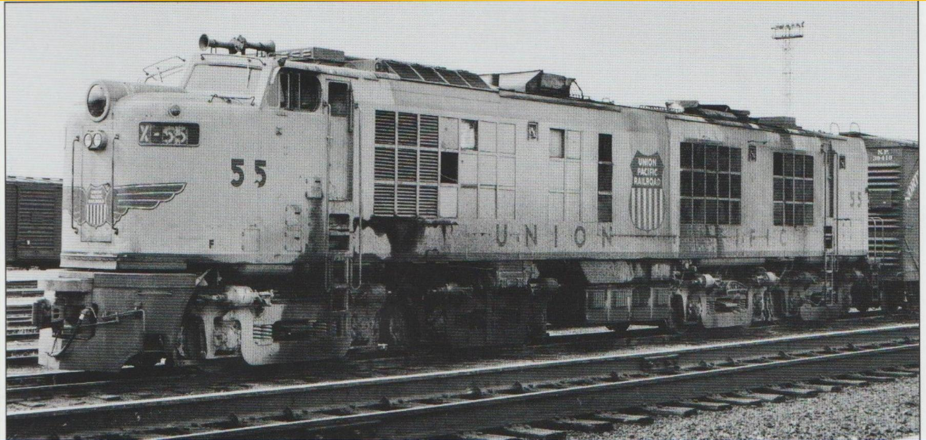
In 1956 the UP began replacing the Farr grilles with louvered air vents as seen behind the cab door.
