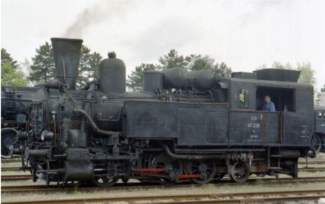
The locomotive, originally designated 69.08 by the kkStB, was based in Vordernberg all its life. It performed the demanding and heavy service on the rack section of the Erzbergbahn. The ÖBB gave it the number 97.208 and equipped it with a Giesl ejector in 1956. At the beginning of 1978 it received a major overhaul and was thus the last standard gauge steam locomotive to undergo this extensive work for scheduled use. It was the last locomotive in its series to be decommissioned in 1978.
