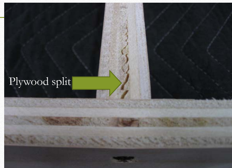
Very weak joint
